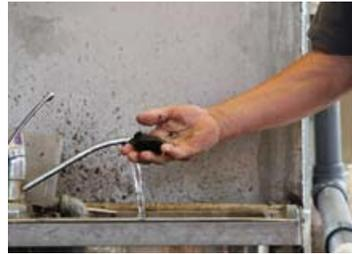
This picture shows checking coagulation or flocculation to monitor polymer dosage. When the water runs clear and the solids stay in a ball means you are at the correct polymer dosage.
